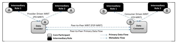
Figure 5: Runtime Environment for Metadata Flow Control based on Data Sharing Connectors.
